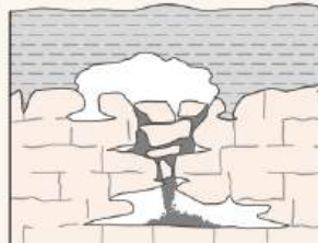
Figure 3-8 Cross section of sinkholes showing both gradual subsidence (Top) and sudden subsidence (Bottom). Sudden subsidence involves the collapse of a void in the surficial cover and is most common in cohesive soils. From Galloway et al. (1999).
