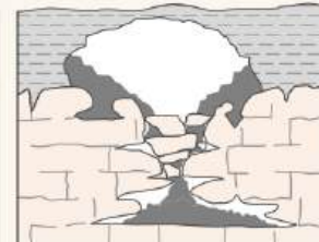
Figure 3-8 Cross section of sinkholes showing both gradual subsidence (Top) and sudden subsidence (Bottom). Sudden subsidence involves the collapse of a void in the surficial cover and is most common in cohesive soils. From Galloway et al. (1999).
