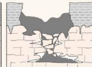
Figure 3-8 Cross section of sinkholes showing both gradual subsidence (Top) and sudden subsidence (Bottom). Sudden subsidence involves the collapse of a void in the surficial cover and is most common in cohesive soils. From Galloway et al. (1999).
